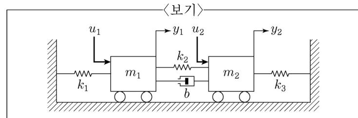
$$\textcircled{1} \quad \begin{bmatrix} \dot{x}_1 \\ \dot{x}_2 \\ \dot{x}_3 \\ \dot{x}_4 \end{bmatrix} = \begin{bmatrix} 0 & 1 & 0 & 0 \\ -k_1/m_1 & -b/m_1 & k_2/m_1 & b/m_1 \\ 0 & 0 & 0 & 1 \\ k_2/m_2 & b/m_2 & -k_2-k_3/m_2 & -b/m_2 \end{bmatrix} \begin{bmatrix} x_1 \\ x_2 \\ x_3 \\ x_4 \end{bmatrix} + \begin{bmatrix} 0 & 0 \\ 1/m_1 & 0 \\ 0 & 0 \\ 0 & 1/m_2 \end{bmatrix} \begin{bmatrix} u_1 \\ u_2 \end{bmatrix}$$
