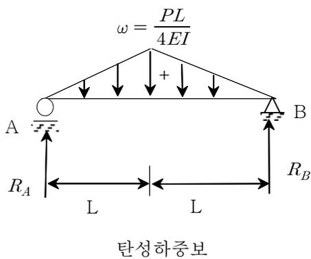
$$\theta_{\max} = \theta_A = S_A = R_A = \frac{1}{2} \times \left( \frac{1}{2} \times 2L \times \frac{PL}{4EI} \right) = \frac{PL^2}{8EI}$$
