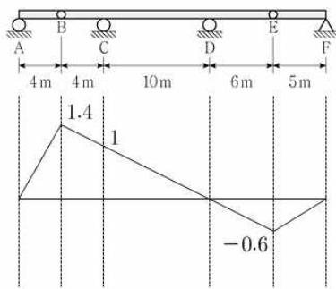
$$\therefore R_{c-\max} = 1.4 \times 30kN = 42kN$$
