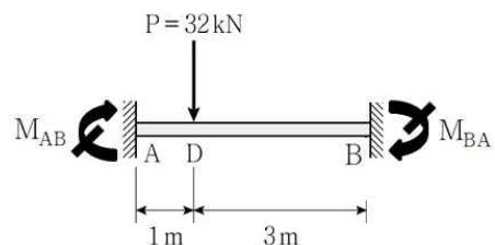
$$M_{AB} = -\frac{(32kN)(3m)^2(1m)}{(4m)^2} = -18kN \cdot m$$
