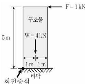
$$\textcircled{1} \text{ 외력 모멘트} : M_d = F \times 5m = 1kN \times 5m = 5kN \cdot m$$
