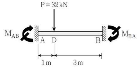
$$M_{AB} = -\frac{(32\text{kN})(3\text{m})^2(1\text{m})}{(4\text{m})^2} = -18\text{kN} \cdot \text{m}$$
