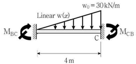
$$M_{BC} = -\frac{(30\text{kN/m})(4\text{m})^2}{30} = -16\text{kN} \cdot \text{m}$$
