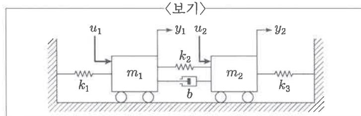
$$\textcircled{1} \quad \begin{bmatrix} \dot{x}_1 \\ \dot{x}_2 \\ \dot{x}_3 \\ \dot{x}_4 \end{bmatrix} = \begin{bmatrix} 0 & 1 & 0 & 0 \\ -k_1 & -b & k_2 & b \\ m_1 & m_1 & m_1 & m_1 \\ 0 & 0 & 0 & 1 \end{bmatrix} \begin{bmatrix} x_1 \\ x_2 \\ x_3 \\ x_4 \end{bmatrix} + \begin{bmatrix} 0 & 0 \\ \frac{1}{m_1} & 0 \\ 0 & 0 \\ 0 & \frac{1}{m_2} \end{bmatrix} \begin{bmatrix} u_1 \\ u_2 \end{bmatrix}$$
