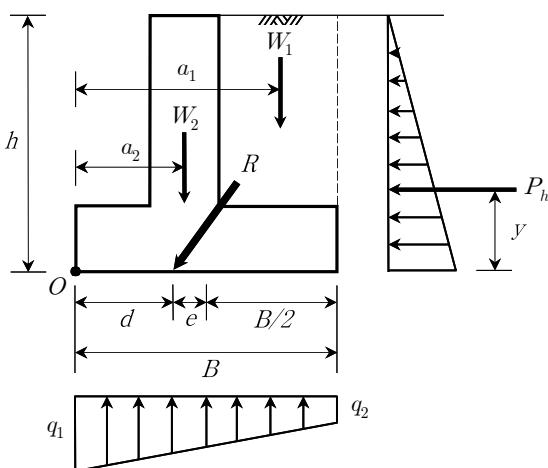
$$\textcircled{1} \quad \Sigma W = W_1 + W_2, \quad \Sigma H = P_h, \quad \Sigma M_r = W_1 a_1 + W_2 a_2,$$
